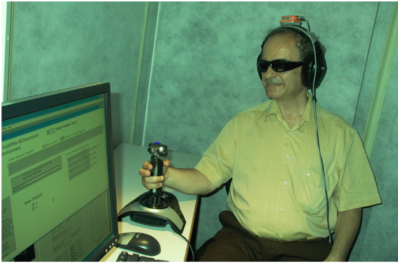
Fig. 4. Blind individual performing virtual navigation using the joystick and wearing headphones equipped with orientation sensor. The screen provided feedback for the operator.
